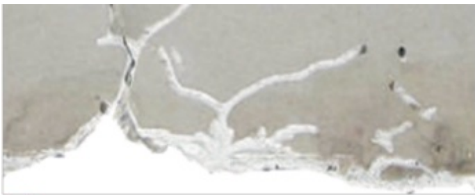
❌ Example: Gypsum Board Not termite resistant
